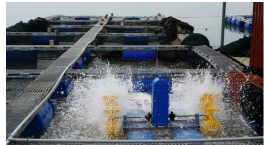
Figure 2: One of the methods of increasing the Dissolved Oxygen level by using paddle wheels
