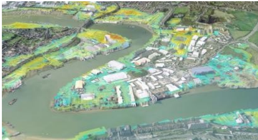
Fig.8 DEM of flood depth and extent map
