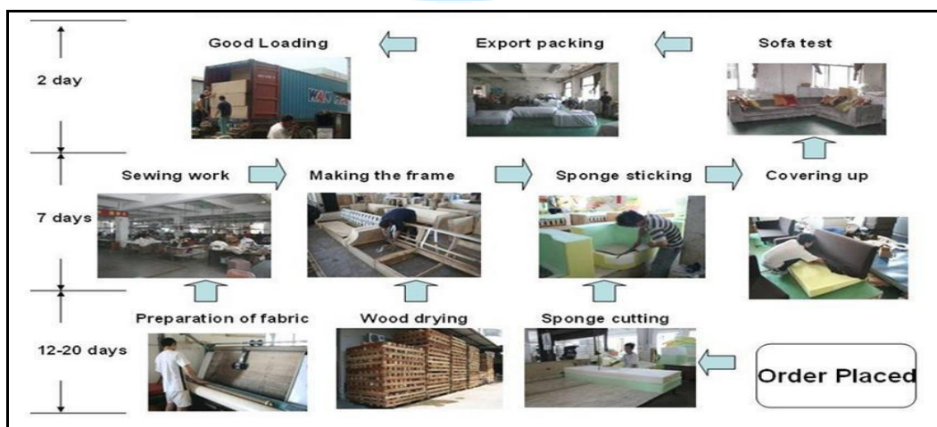
Figure 3 : Sofa Development Process / Gambarajah 3: Proses Pembangunan Sofa (Sumber : Thai Furniture Industries Association, Thai Furniture Exports, available online at www.tfa.co.th/Th/_tfa/newsfile/thaifurnitureexport_(dec.).pdf , accessed on April 2011)
