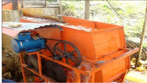
Figure 5. 3 KW Overshoot Water Wheel Generator
