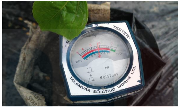
Figure 3.9: Reading of soil moisture and soil pH by using soil tester
