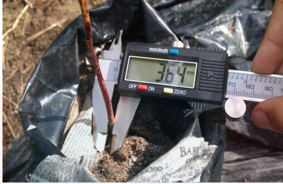
Figure 3.11: Measuring diameter of stem by using Vernier caliper
