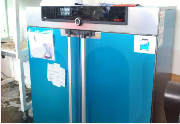
Figure 3.12: Used oven to drying stems, roots, and fruit about 48 hours in 65°C
