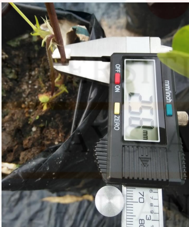
Figure A2: The diameter of stem was measured by using digital calliper
