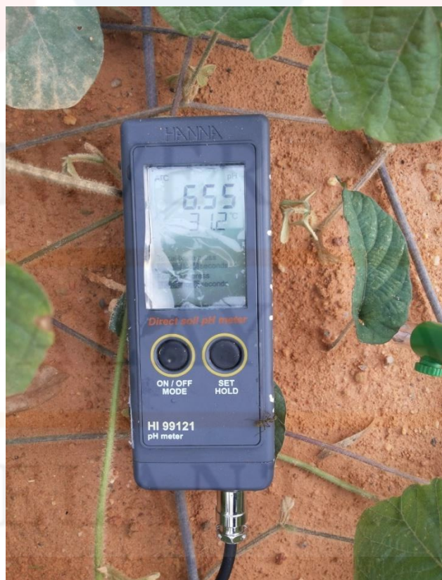
Figure D.4: Soil pH Meter to determine the pH of Red Soil at AgroPark UMK Jeli.
