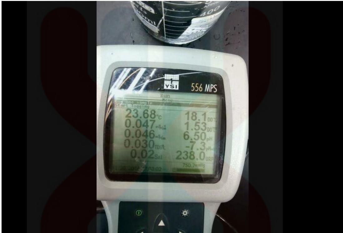
Figure E.1: YSI Multiparameter to Determine the Physical and Chemical Properties of Water Sample.
