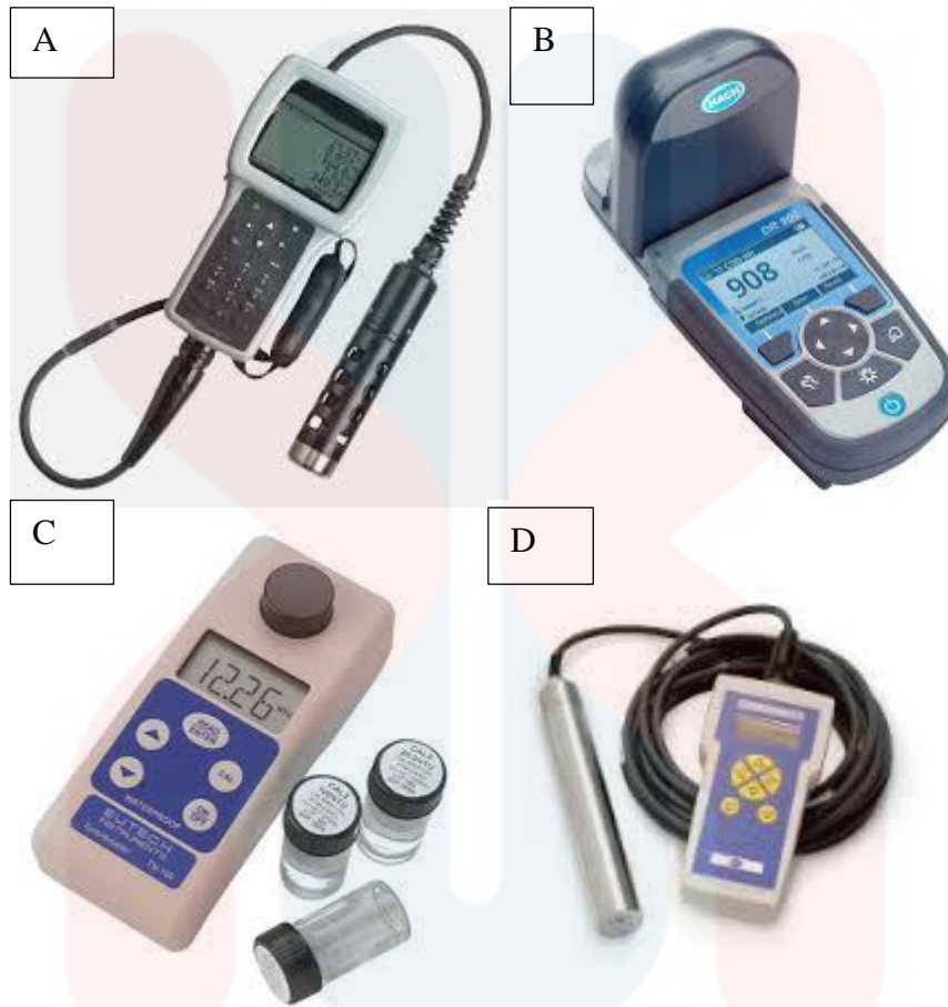
Figure 6.0 : In- Situ parameter instruments. (A) Portable Total Dissolved Solid, (B) Calorimeter, (C) Turbidimeter, (D) Portable Total Suspended Solid.
