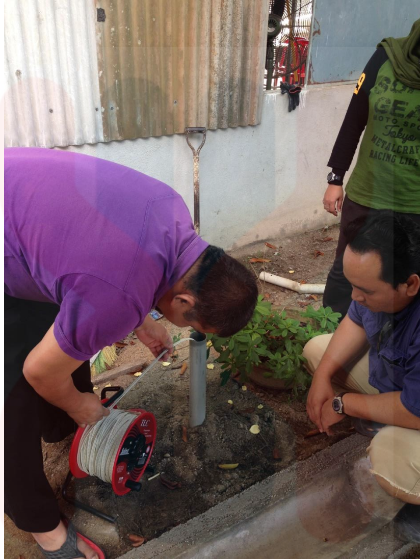
Figure 3.16: Measure the depth of water and well
