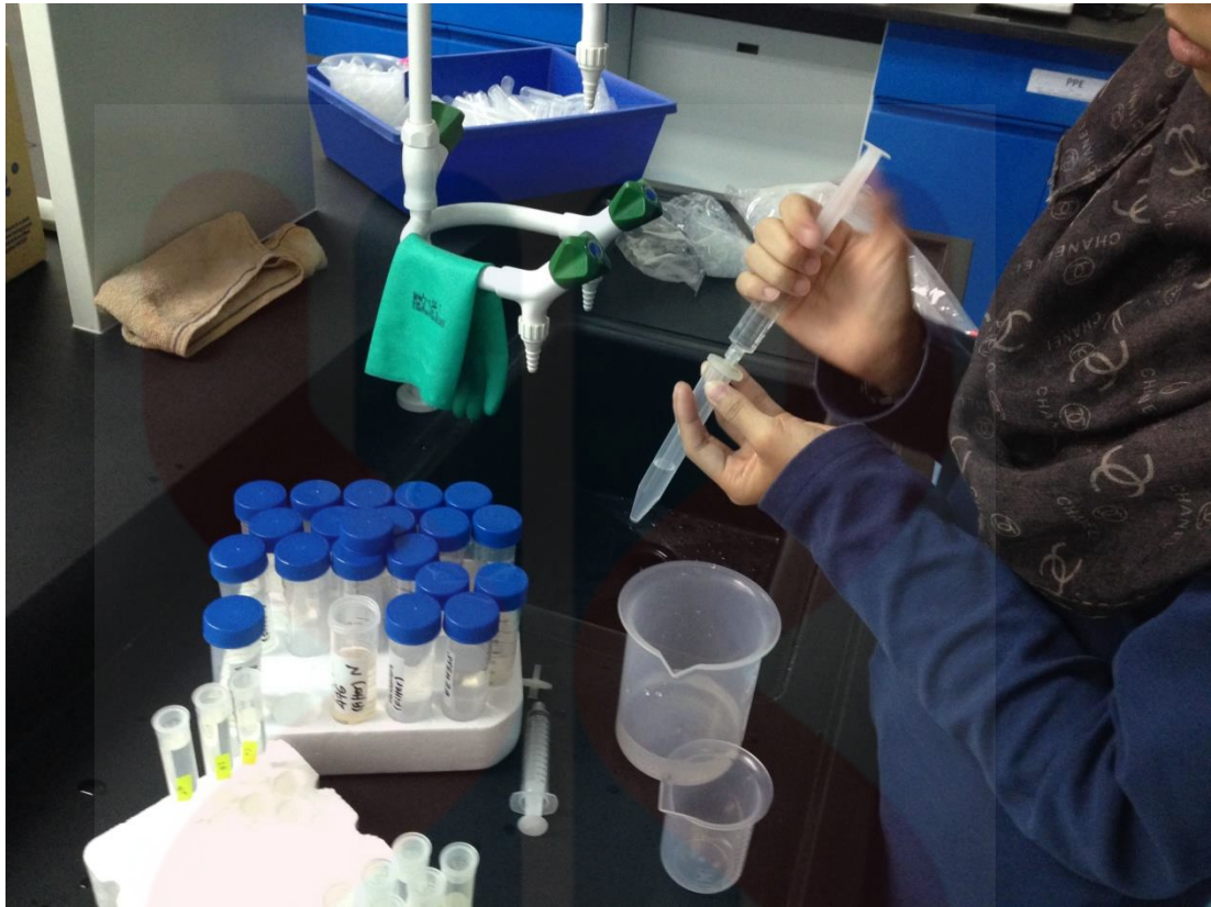
Figure 3.19: Purifying the sample before run the IC method.
