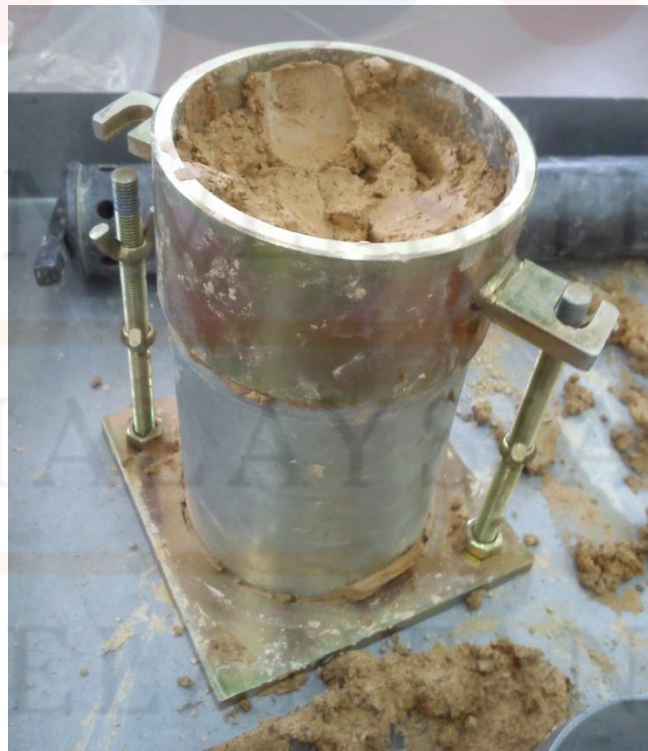
Figure 3.3: Soil compaction for permeability test
