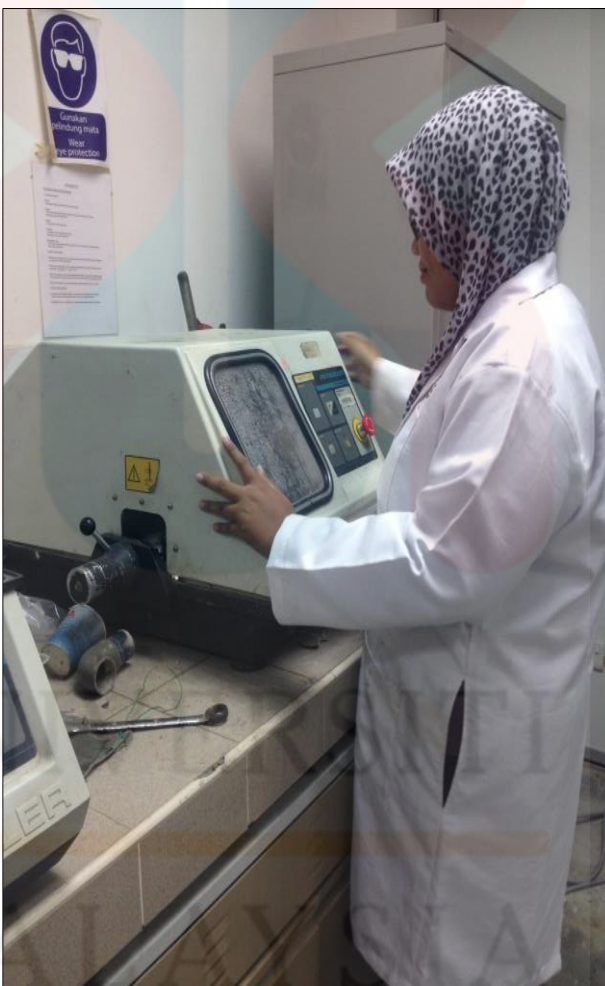
Figure 3.3 shows the cutting of rocks using The Diamond Slab Saw machine
