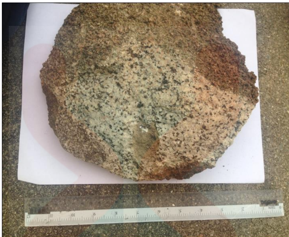
Figure 4.25 : The hand specimen of granite at station 4
