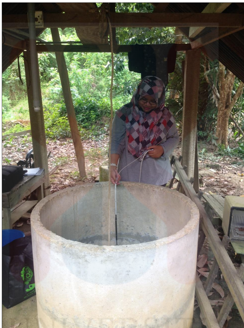
Figure 5.6 shows the measurement of well water depth
