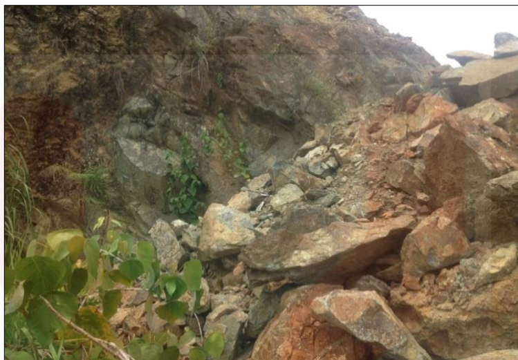
Figure 4.12 :The result of physical weathering where some of the rocks were broken into smaller size
