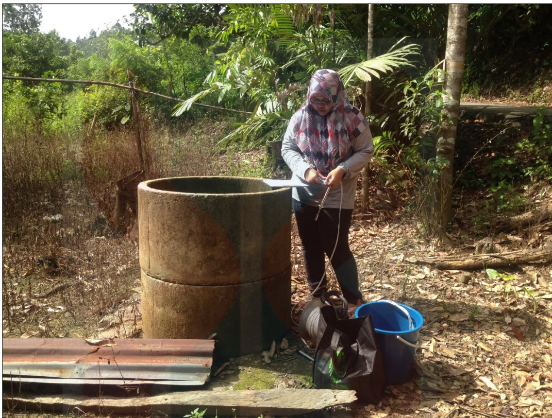
Figure 5.5 shows the measurement of water level depth using water depth meter
