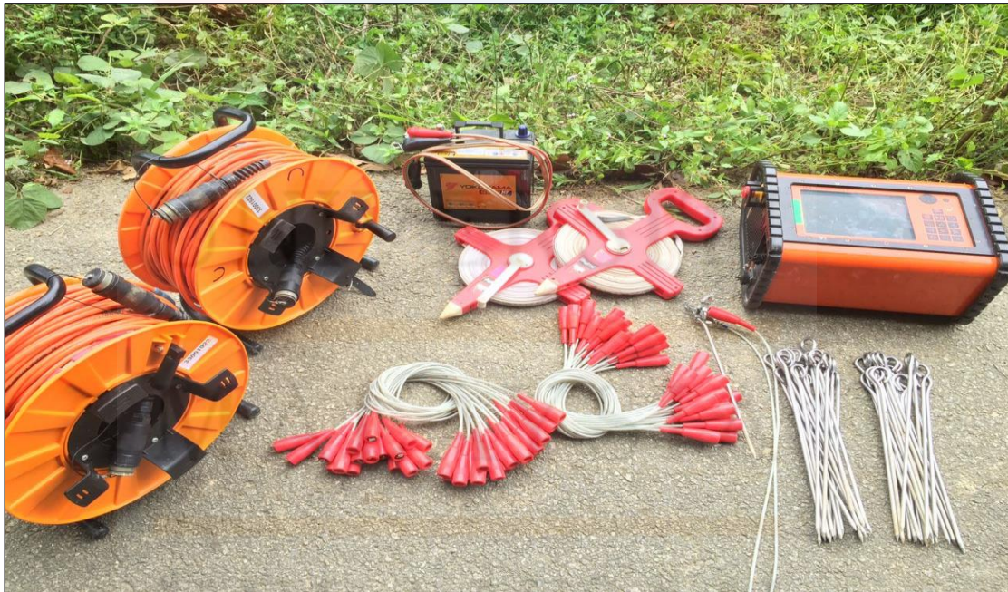
Figure 5.1 : The instruments of the electrical resistivity method
