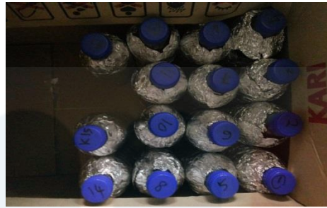
Figure 3.4: Shows the water sampling wrapped with aluminium foil.
