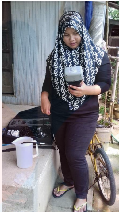
Measure the reading of water using Multipara meter.
