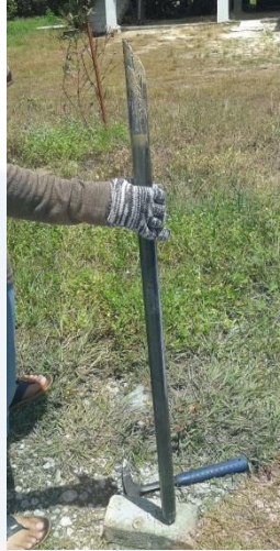
Figure 3.2: The auger that used in alluvium mapping.
