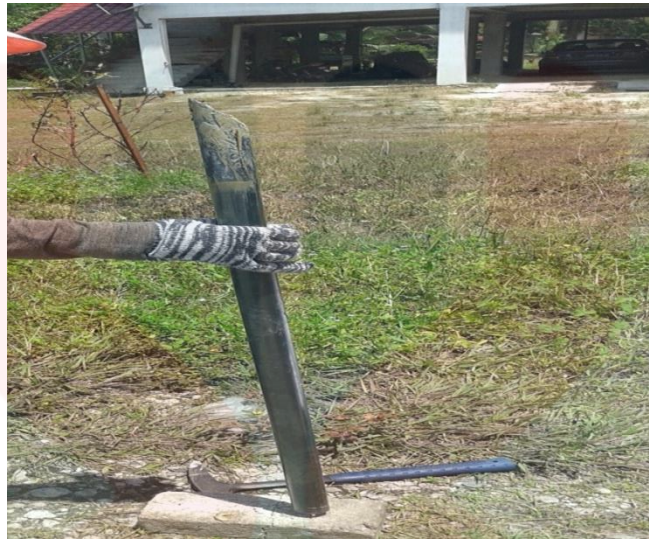
Soil sampling using auger.
