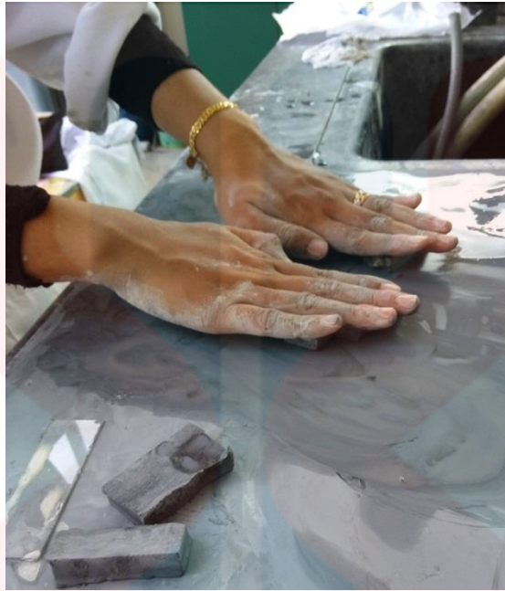
Figure a: The slide was rubbed using carbon to frost the slide surface
