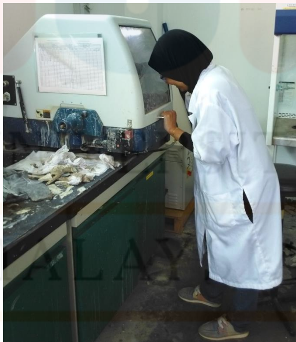
Figure b: The rock was cut by using the slab saw
