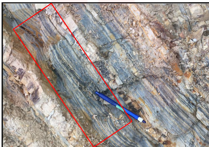
Figure 5.5 shows wavy bedding between sandstone and mudstone strata
