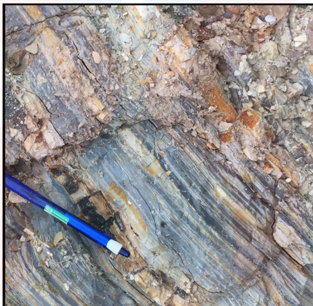
Figure 5.4: Lamination in shale bed with thickness of 3mm to 9 mm.
