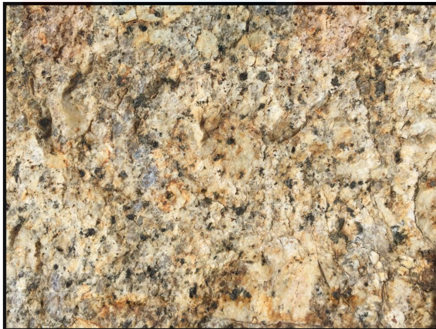
Figure 4.13 shows the volcanic sandstone comprised with sand-sized grain
