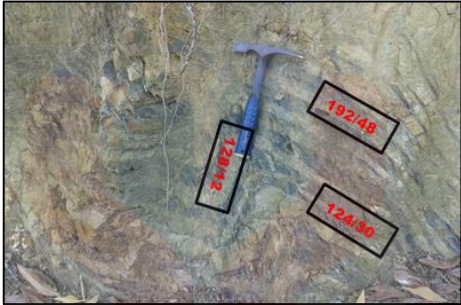
Figure 4.19: The overturned fold with the reading of strike and dip
