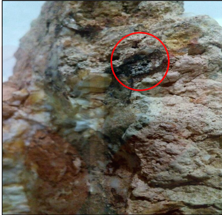
Figure 4.5: Chemical weathering that cause the iron stain appears on rocks.
