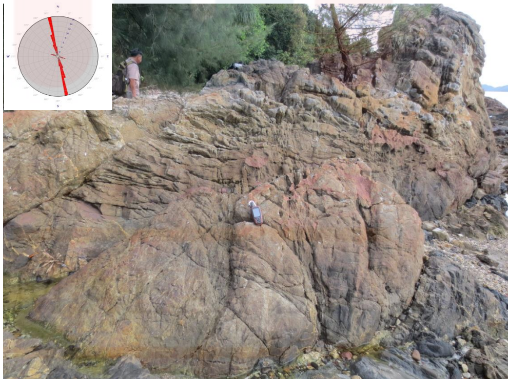
Figure 4.45: The sandstone body with azimuth of 92° N that has systematic joints with rose diagram that shows the direction of maximum forces ( \sigma_1 ) comes from SE 165°.
