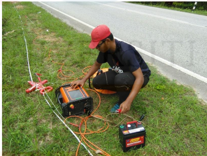
Figure B.6 Setup resistivity machine (Abem Terrameter)
