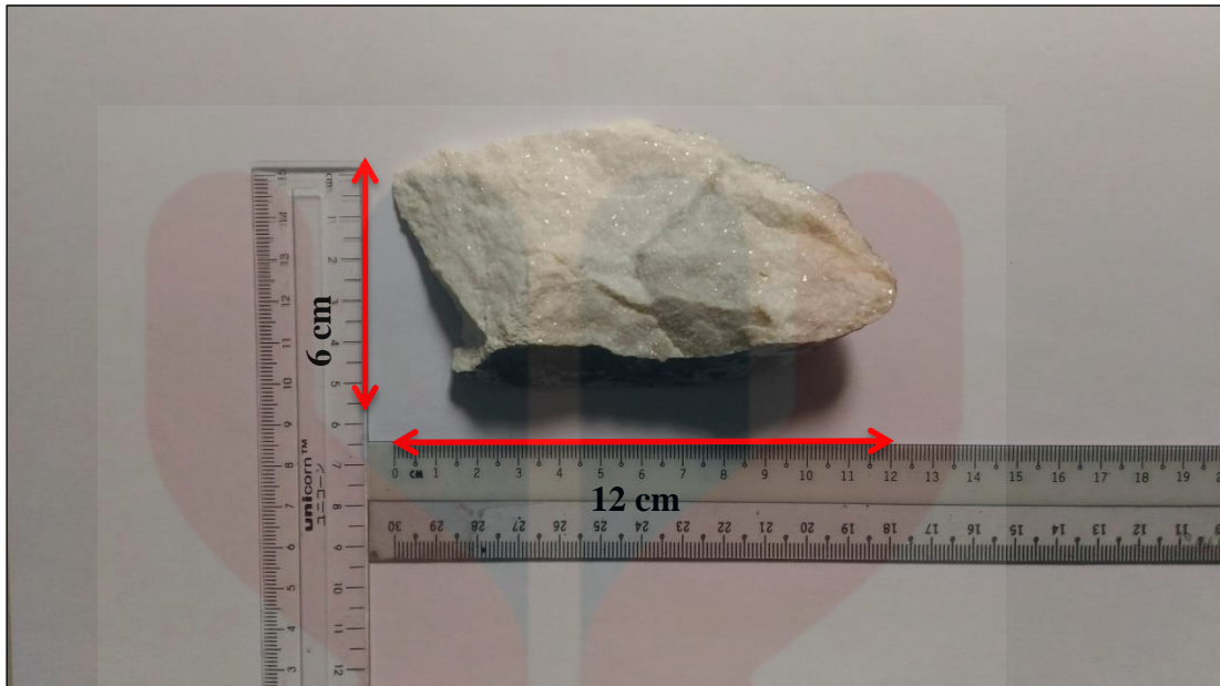
Figure 4.18: Hand specimen of marble with scale
