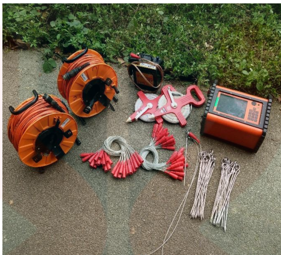
Figure 3.2: Image of resistivity measurement equipment
