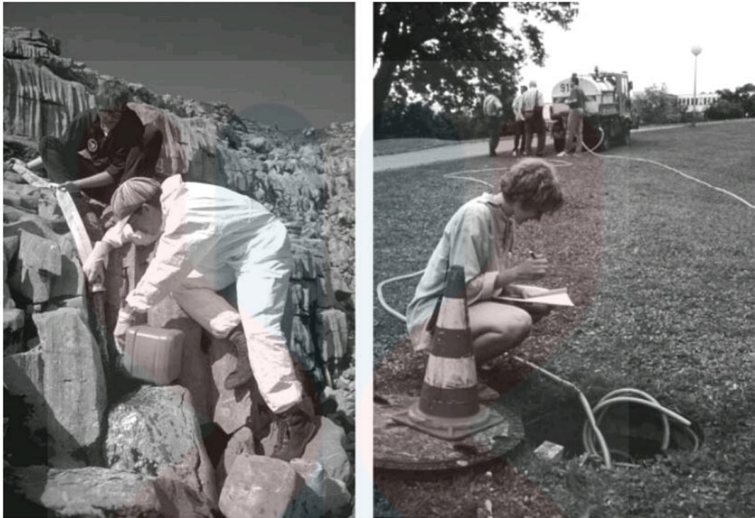
Figure 2.2: Left: Injection of of uranine from a plastic container into a karst shaft. Right: Injection of naphthionate, dissolved in a tank, into an observation well in the confined karst aquifer of a mineral springs (Nico Goldscheider, 2007).
