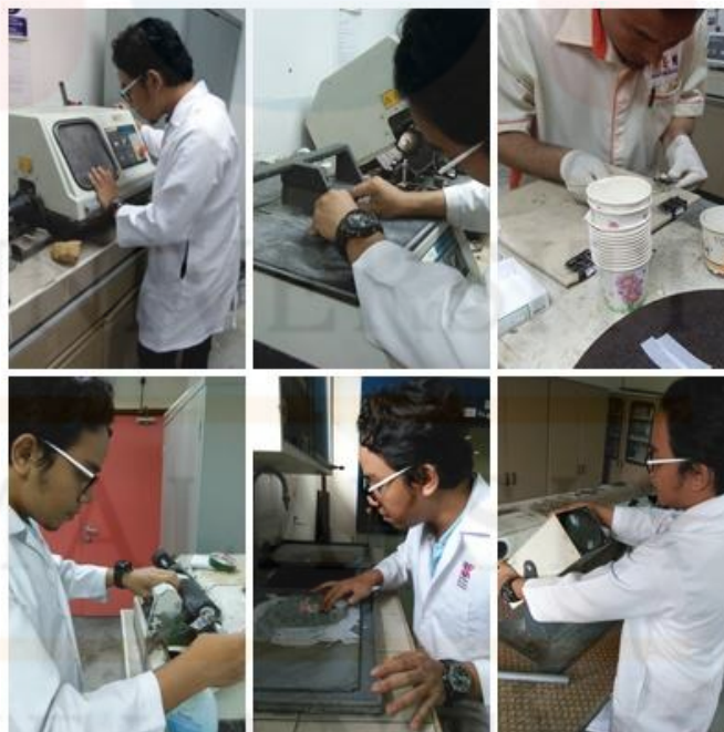
Figure 7.4: Thin section preparation. 1) Cut the sample into smaller size. 2) Cut the sample into fitting size for the slide. 3) Glue the sample into the slide. 4) Thinning the sample. 5) Smooth the sample surface. 6) Check for observable mineral or repeat Process 4 and 5.
