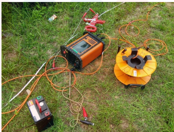
Figure 3.1: ABEM Terrameter S4000 and related equipment for ERI survey
