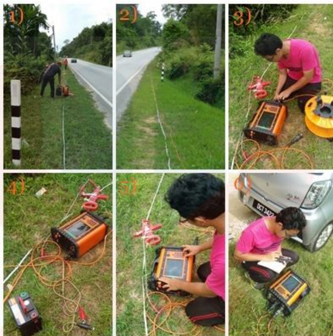
Figure 7.3: Procedure for ERI survey. 1) Choose suitable location with straight survey line. 2) Set up the electrode. 3) Connect the wire. 4) Put on the battery. 5) choose the array and let it run until it stop. 6) Record necessary data and pack up.
