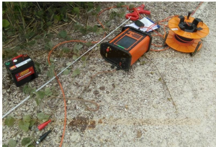
Figure 5.1: ABEM Terrameter S4000 and related equipment for ERI survey.
