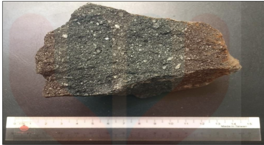
Figure 4.18 Hand specimen on tuff in Volcanic Product of Putri – Katomas (P-K v )
