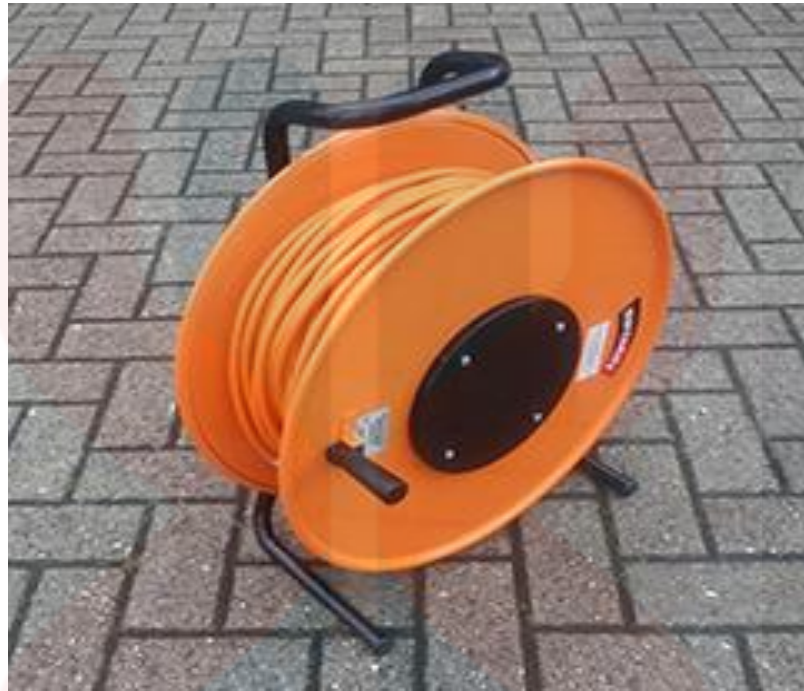
Figure 5.3 Resistivity Cable (100 meter)
