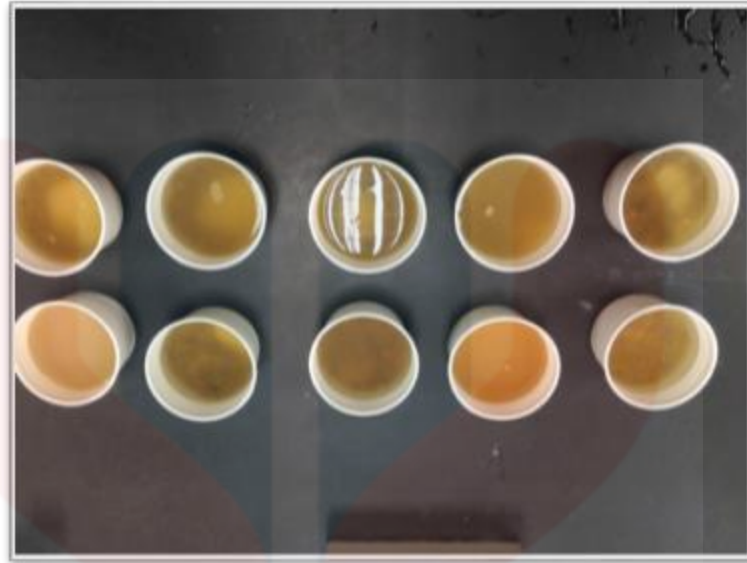
Figure 3.5: Stream sediments left overnight with 100ml of distilled water
