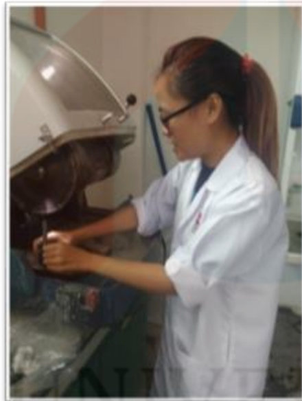
Figure 3.8: Sectioning rock process
