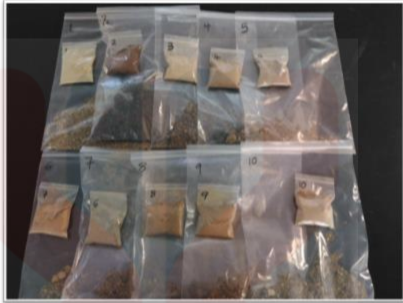
Figure 3.4: Prepared samples to be sent to the lab for XRF analysis
