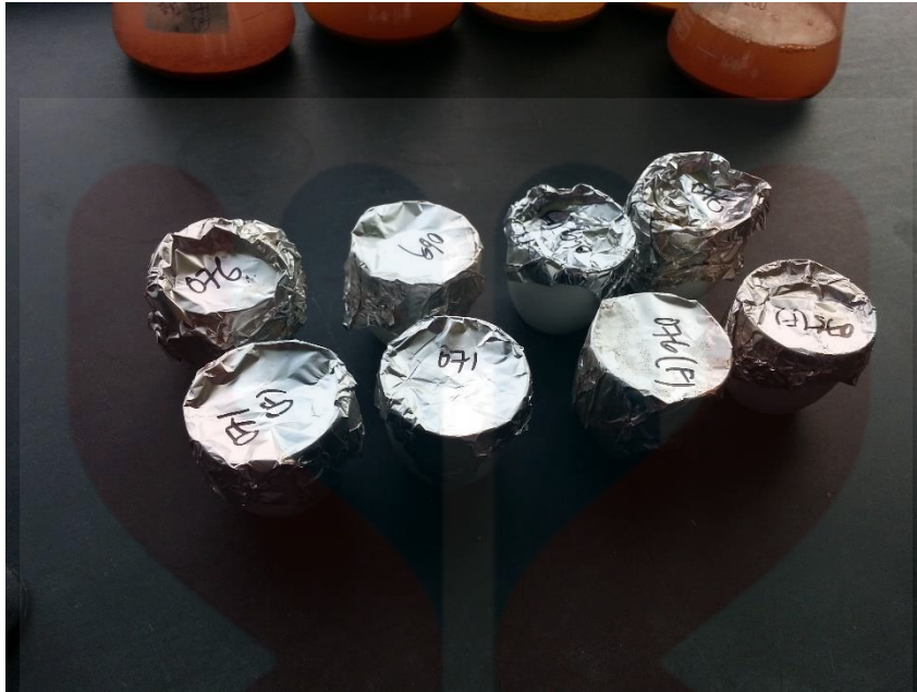
Photo F5: Soil sample from plastic limit test
