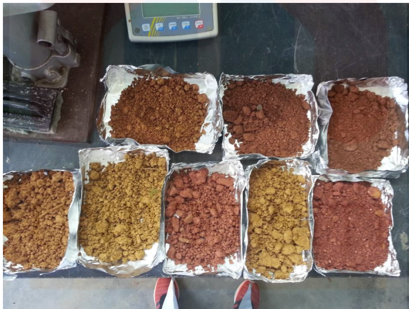
Photo F2: Moisture content laboratory test
