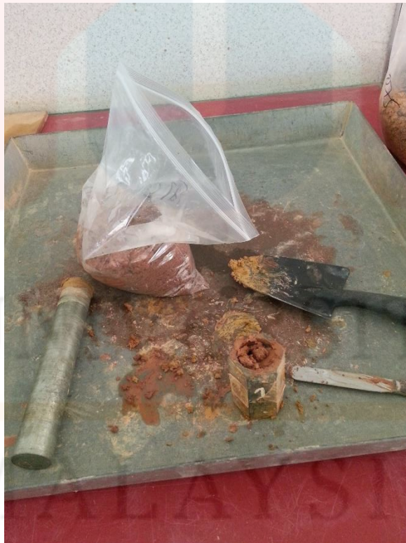
Photo F6: Soil sample preparation for vane shear strength test
