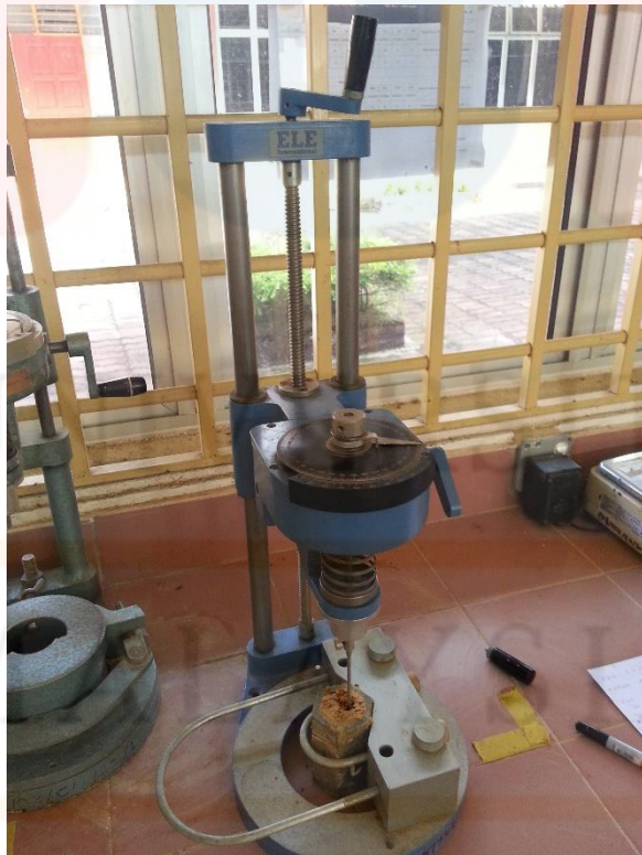
Photo F8: Laboratory vane shear strength test (Test at Politeknik Kota Bharu)
