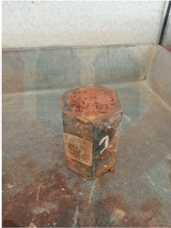
Photo F7: Soil sample for vane shear strength test
