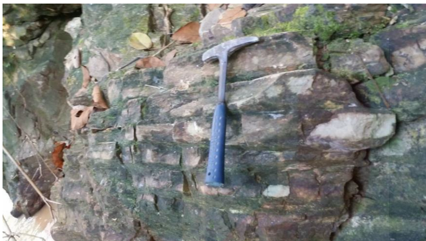
Figure 4.20(a): Bedding of sandstone
