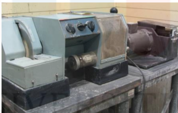
Figure 3.8: Dual and single blade rock saws for cutting samples to the required size
