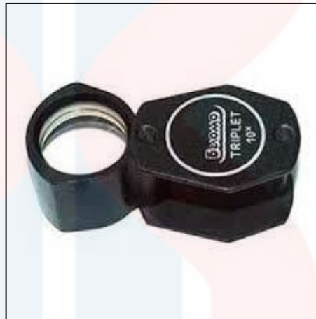
Figure 3.5 : A 10x hand lens
