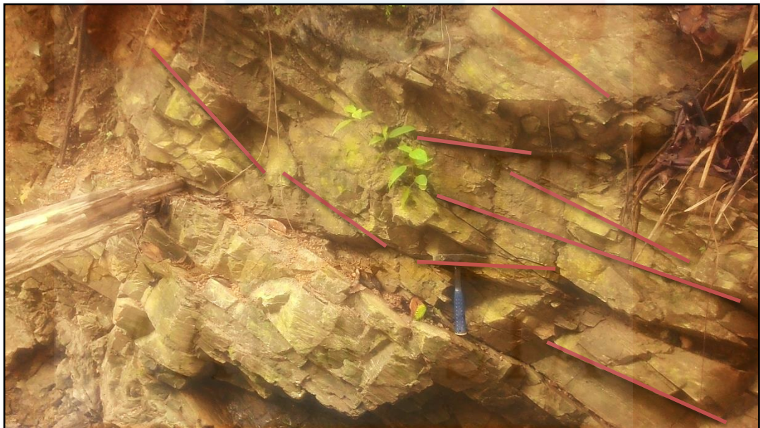
Figure 5.6 : The shear and extensional joint on sandstone outcrop.
