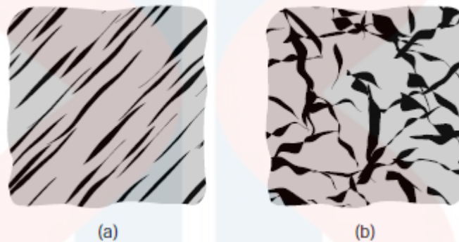
Figure 2.8 : The types of vein arrays. Vein fill is dark (a) Planar array of veins. (b) Stockwork array of veins. (source : Van Der Pluijm, Ben A., 2004)
