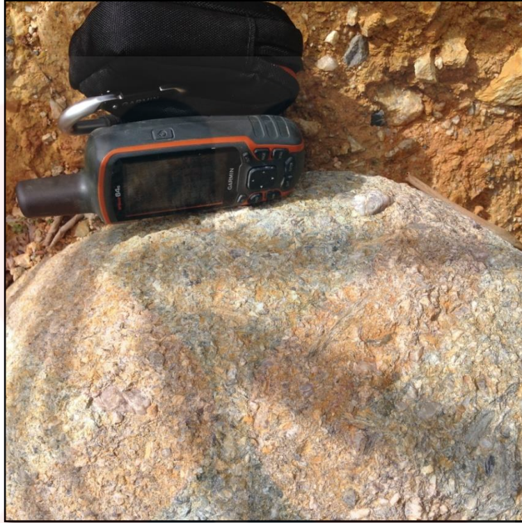
Figure 4.24 : The conglomerate with clasts range from 5 mm to 30 mm, GPS act as scale.
