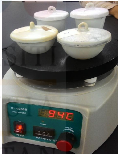
Figure A. 8: The combustion process to measure soil organic matter.
