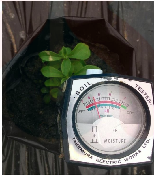
Figure 3.5: soil tester was used as to measure the soil moisture and pH.
