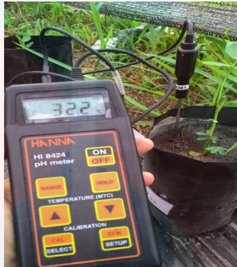
Figure 3.3: pH meter as measure the temperature of soil
