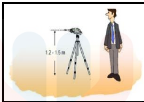
Figure 3.6: Sound level meter mounted on tripod (Kjaer, 2000).
