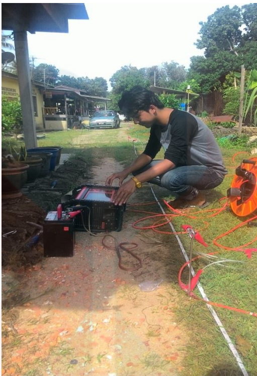
Figure B1: ABEM Terrameter Resistivity Test
