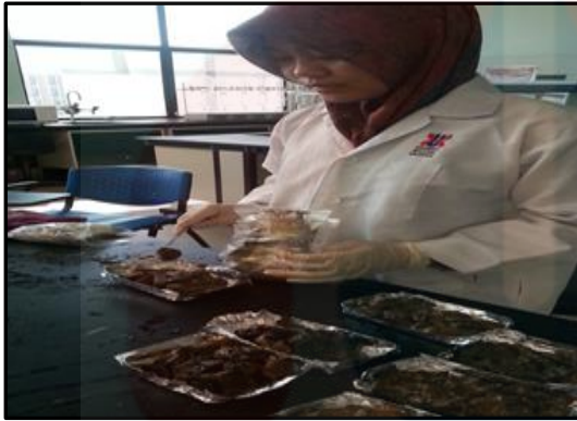
Figure B.3: Sediment samples were categorized before was put in Drying Oven for 105°C (24 hours).
