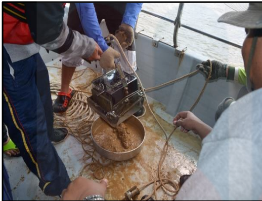
Figure B.1: 4cm of sediment was collected by using Ekman grab
