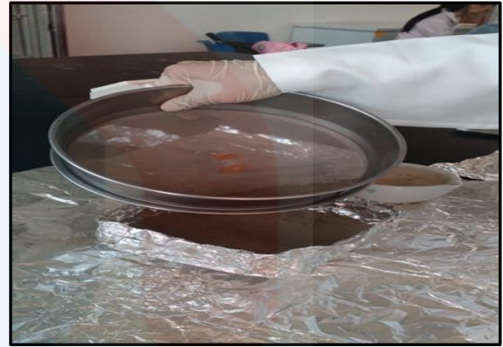
Figure B.4: The samples were sieved by using 75µm sieve
