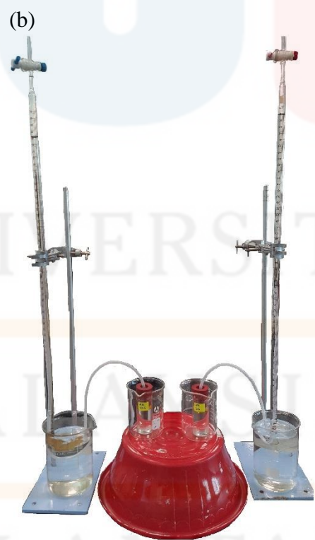
Figure 3.4 Actual experiment setup for volumetric measurement that run for (a) single and (b) multiple evaluation.
