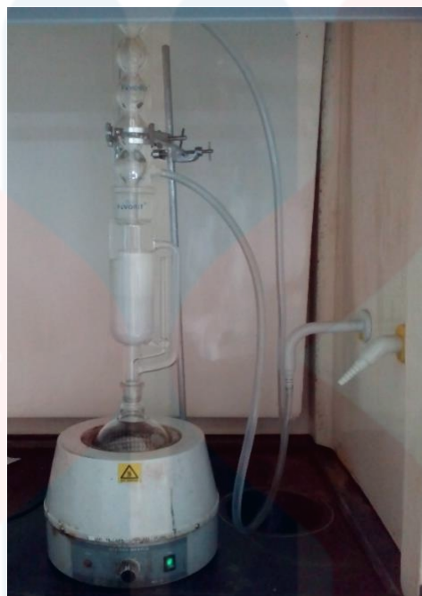
Figure 3.2: The soxhlet apparatus setup
