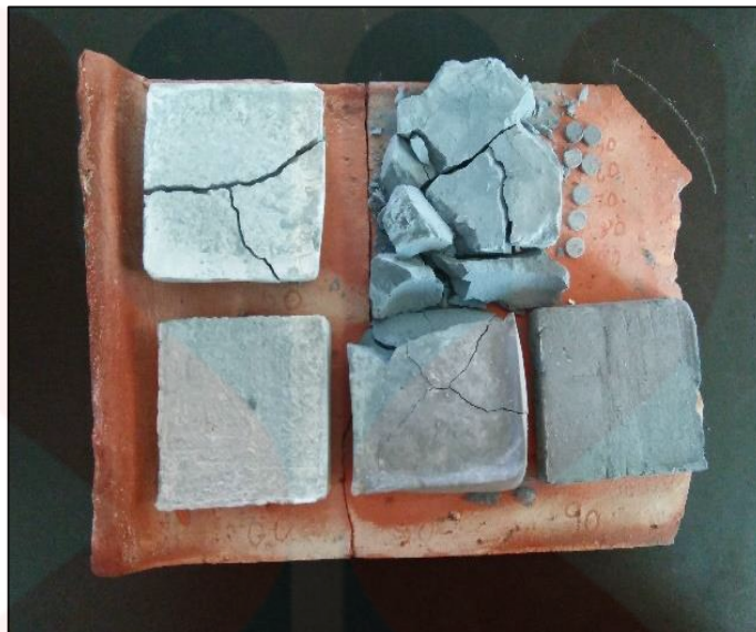
Figure 4.8: The composite after sintering process
