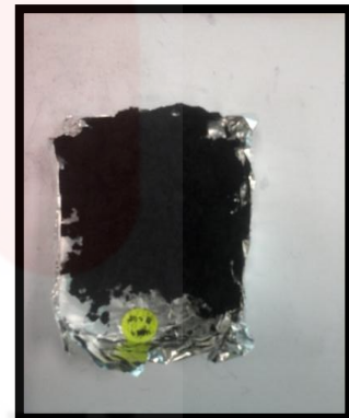
Oven-dried \alpha -cellulose after placed in oven at 60°C for 24hours.
