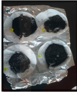
Oven-dried holocellulose of torrefaction sample placed in oven at 70°C for 24hours.
