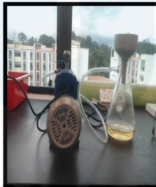
Sample is filter by using bunched funnel and vacuum pump with 250ml cold dH 2 O, 25ml of 8.3% NaOH and 50 ml
