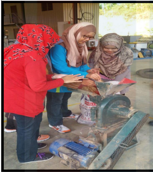
EFB was grinded to reduce the size by using grinder at Agro Park.
