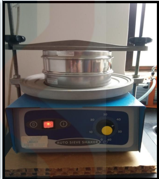
After grinding, the sample was sieve by using a auto sieve shake to get the 500 micron.
