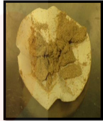
Oven-dried holocellulose of raw sample placed in oven at 70°C for 24hours.
