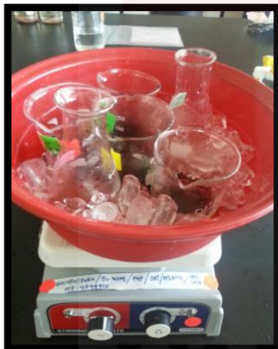
Process to determined \alpha -cellulose by mixing 17.5% NaOH with stirring iced environment due to exothermic nature of reaction acetone
