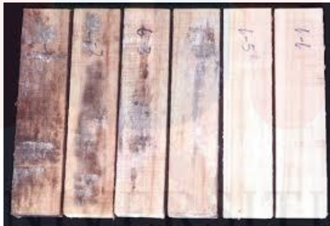
Figure 2.3: Sapstain (or blue stain) on Rubberwood Source: (Teoh et al. , 2011)
