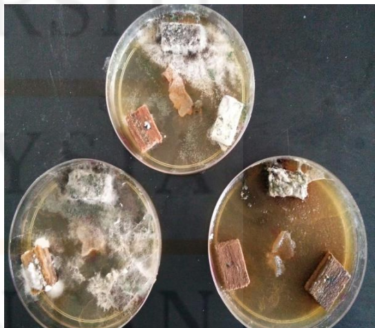
Figure A6: Wood decay fungal test after 1 month
