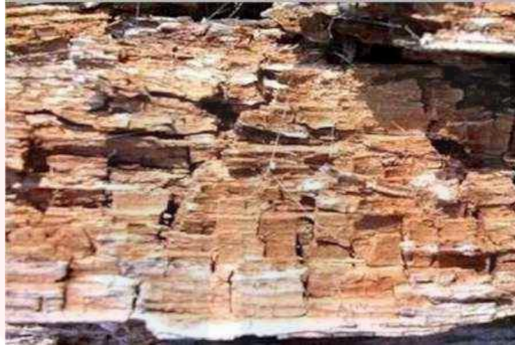
Figure 2.5: Part of a pine stump showing the characteristic brick-like decay by brown-rot fungi.
