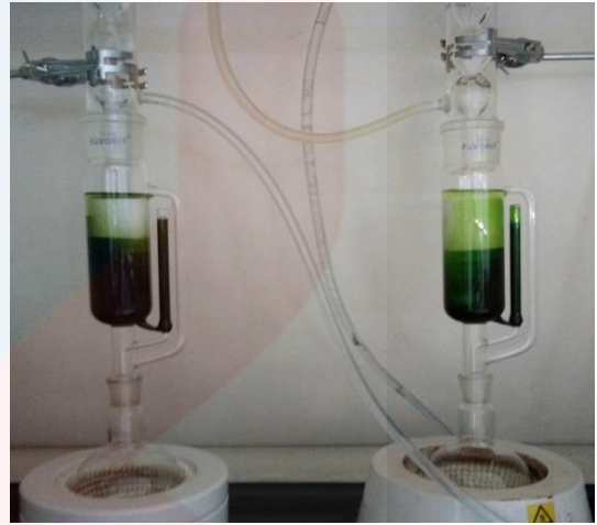
Figure A2: Extraction process by using Soxhlet
