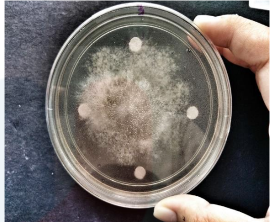
Figure A8: MIC test after 3 days
