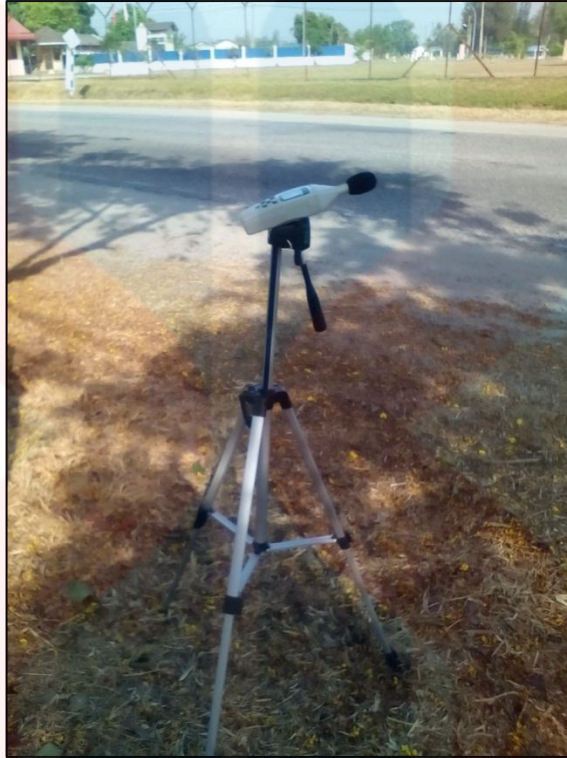
Figure 3.2: The set-up of TENMARS-102 sound level meter
