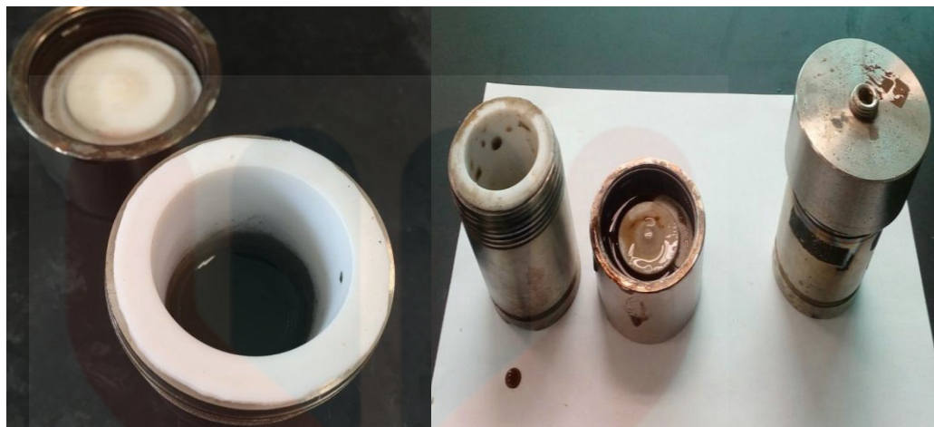
Fig. 3.7 The mixtures is put in the autoclave for hydrothermal treatment
