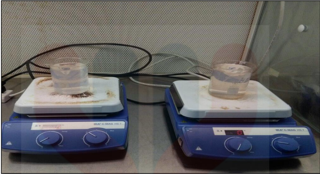
Figure 3.3: Magnetic plate with magnetic stirrer inside each beaker
