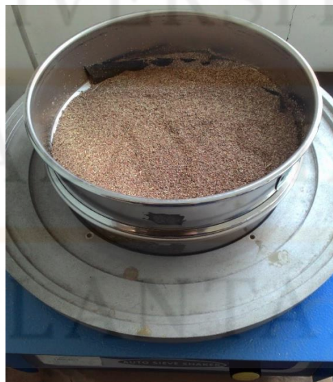
Figure 3.2: The sawdust being sieved by 250\text{ }\mu\text{m} sieve.
