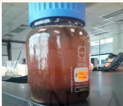
Figure 3.4: The treated sawdust being immersed in distilled water to wash the Ionic liquid.
