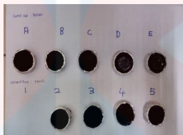
Figure 4.3 Sample for compression testing
