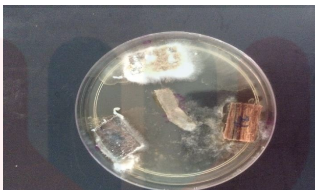
Figure D: Wood decay test after one month
