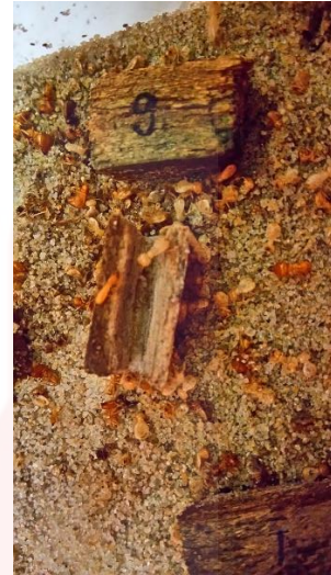
Figure B7: One of the wood being decayed on control specimen
