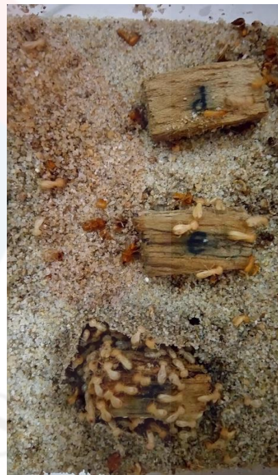
Figure B9: Extractives preservatives on test arena
