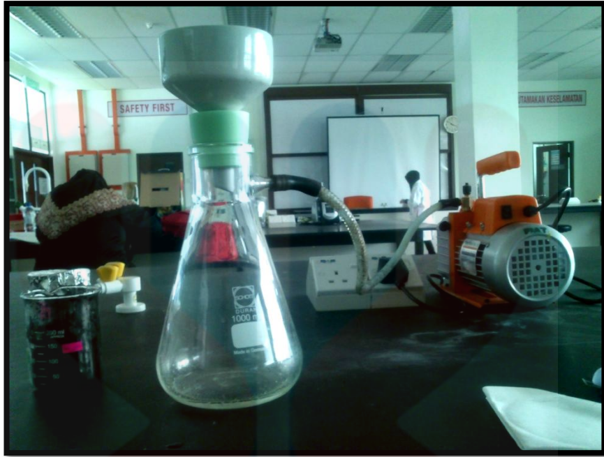
Figure 3: Wash process after soaked with \text{H}_3\text{PO}_4
