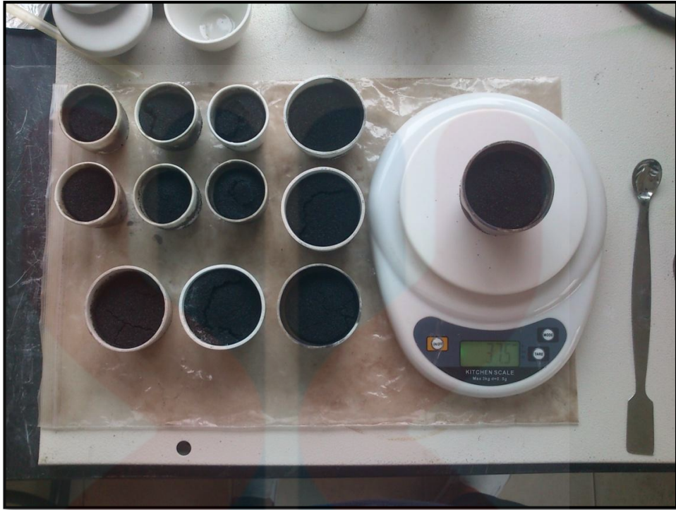
Figure 4.3: Activated carbon of rubber wood sawdust (RWAC)
