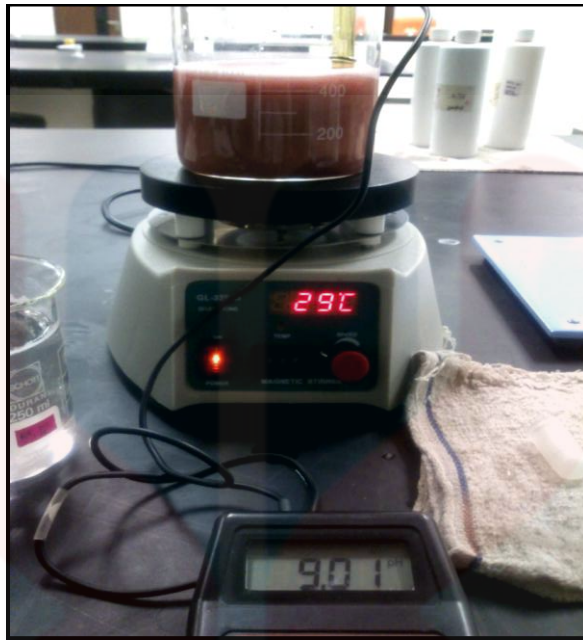
Figure 4.10: The set up for pH altering process
