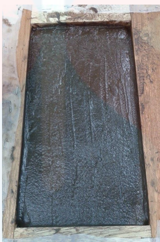
Figure 3.4: The boiled blended mixture was spread over the silk screen in the mould.
