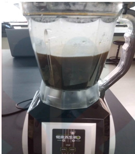
Figure 3.4: Banana peel was blended with eggshell powder and glycerol for 10 minutes.
