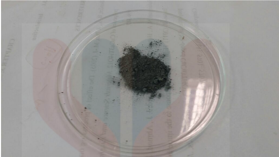
Figure 4.6: CCTO powder after mixing process for 24 hours
