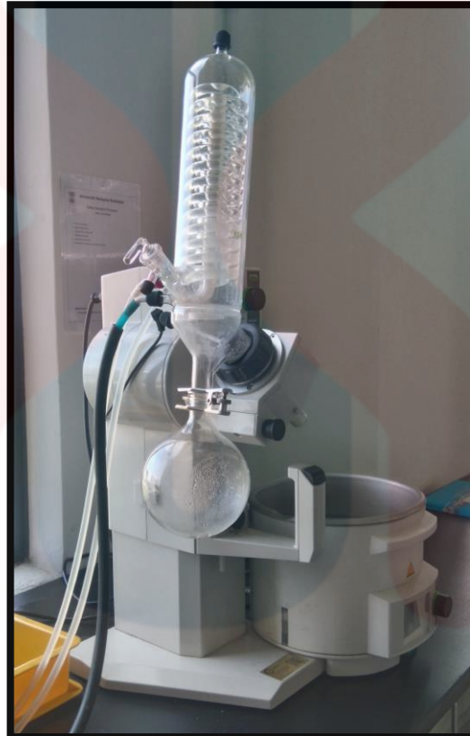
Figure 3.3: The rotaevaporator used in hollow colloidosomes preparation
