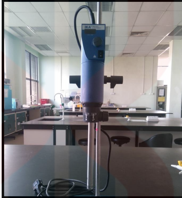
Figure 3.1: Homogenizer used in hollow colloidosomes preparation
