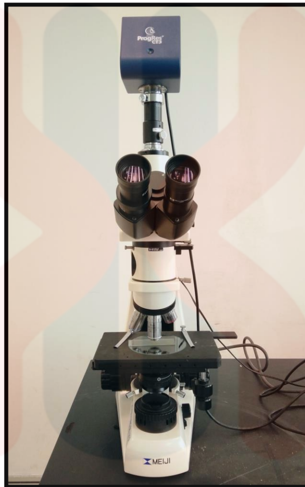
Figure 3.4: An optical microscope used in hollow colloidosomes preparation
