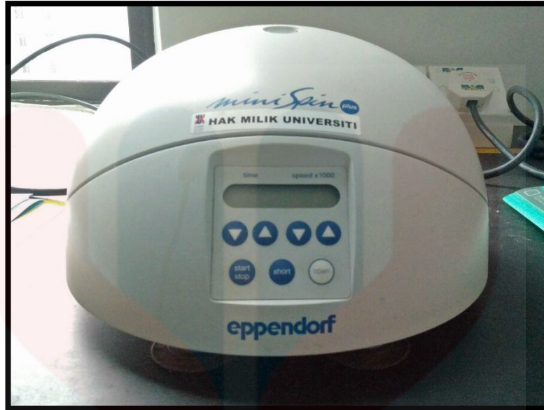
Figure 3.7: The centrifuge used in PCL/PVA hollow colloidosomes preparation
