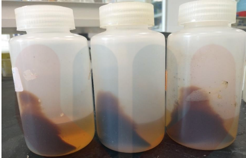
Appendix E: The HA samples that after centrifuged for 15 minutes at 10, 000 rpm.
